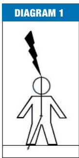
Direct strike with the current passing through the body
